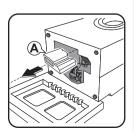
Very carefully remove the front polystyrene block
